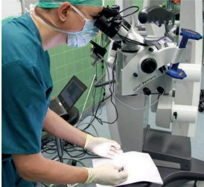
*Figure 4.6: Experimental setup and apparatus used in this study. To our knowledge, this is first time that ones record eye movements under microscope. Through iterative cycles of design, implementation, and evaluation we embedded our eye tracker into a Zeiss neurosurgical microscope (OPMI Pentero). The current version of the prototype is fully functional and complies with the design specifications defined in this study. Reprinted from P (IV).*
